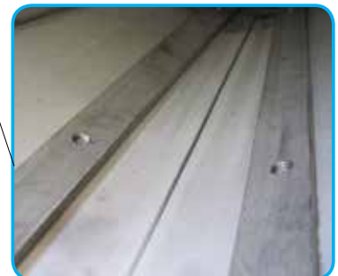
Bolted wear bars (internal view of trough)
