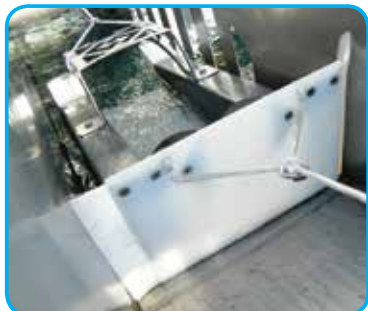
Self-adjusting grease scraper with limited water removal
